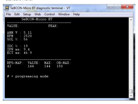
AMM: Voltage of the air mass meter up to max. 5.50 volts
